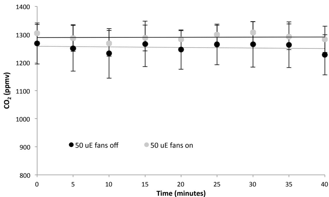
Figure 12: Sealed room trials of CO<sub>2</sub> draw down (as ppmv CO<sub>2</sub> removed) for four modules containing *Epipremnum* at 50  $\mu\text{mol}\cdot\text{m}^{-2}\cdot\text{s}^{-1}$ , with module fans off (dotted line) and running at full output (3.5 m.s<sup>-1</sup>; solid line). Data are corrected for chamber losses ('leakage'). Data are means  $\pm$  SE, n = 3.
