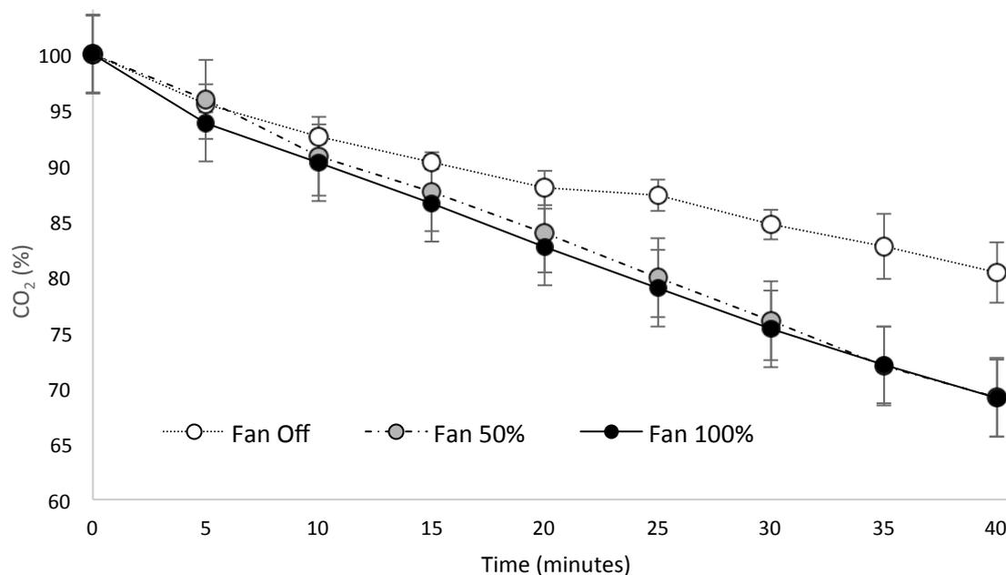
Figure 6: Chamber trials of CO<sub>2</sub> draw down (as % of a starting concentration of ~1000 ppmv) for *Epipremnum* at 100  $\square$  mol.m<sup>-2</sup>.s<sup>-1</sup>, with module fans off, running at full output (3.5 m.s<sup>-1</sup>) and half full output (1.75 m.s<sup>-1</sup>). Data are corrected for chamber losses (leakage). Data are means  $\pm$  SE, n = 3.
