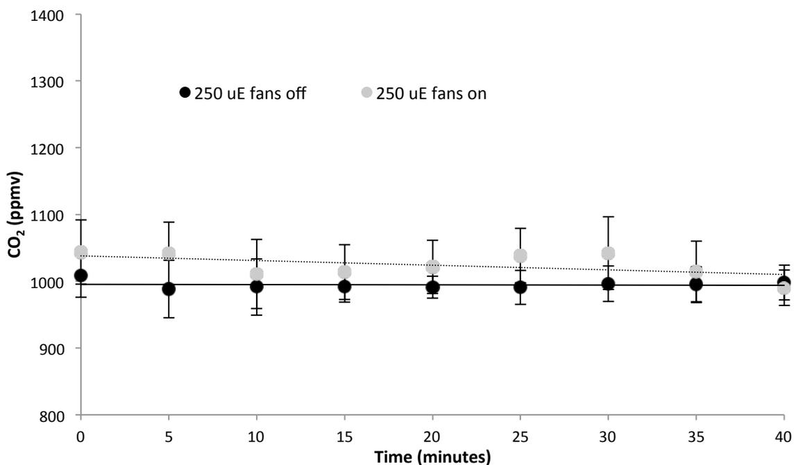
Figure 14: Sealed room trials of CO<sub>2</sub> draw down (as ppmv CO<sub>2</sub> removed) for four modules containing *Epipremnum* at 250  $\mu\text{mol}\cdot\text{m}^{-2}\cdot\text{s}^{-1}$ , with module fans off (dotted line) and running at full output (3.5  $\text{m}\cdot\text{s}^{-1}$ ; solid line). Data are corrected for chamber losses ('leakage'). Data are means  $\pm$  SE, n = 3.
