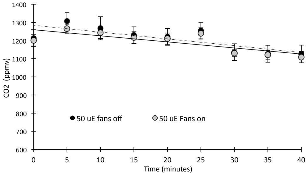
Figure 8: Sealed room trials of CO<sub>2</sub> draw down (as ppmv CO<sub>2</sub> removed) for four modules containing *Chlorophytum* at 50  $\mu\text{mol}\cdot\text{m}^{-2}\cdot\text{s}^{-1}$ , with module fans off (solid line) and running at full output (3.5 m.s<sup>-1</sup>; dotted line). Data are corrected for chamber losses ('leakage'). Data are means  $\pm$  SE, n = 3.
