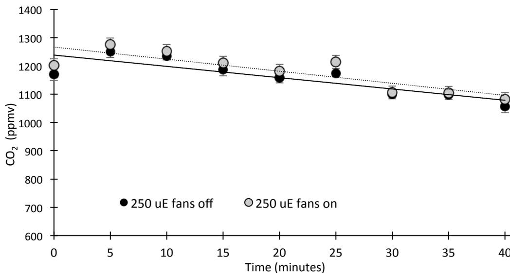
Figure 10: Sealed room trials of CO<sub>2</sub> draw down (as ppmv CO<sub>2</sub> removed) for four modules containing *Chlorophytum* at 250  $\mu\text{mol}\cdot\text{m}^{-2}\cdot\text{s}^{-1}$ , with module fans off (solid line) and running at full output (3.5 m.s<sup>-1</sup>; dotted line). Data are corrected for chamber losses ('leakage'). Data are means  $\pm$  SE, n = 3.
