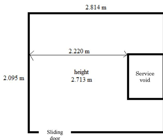
Figure 6: Dimensions of the sealed test room
