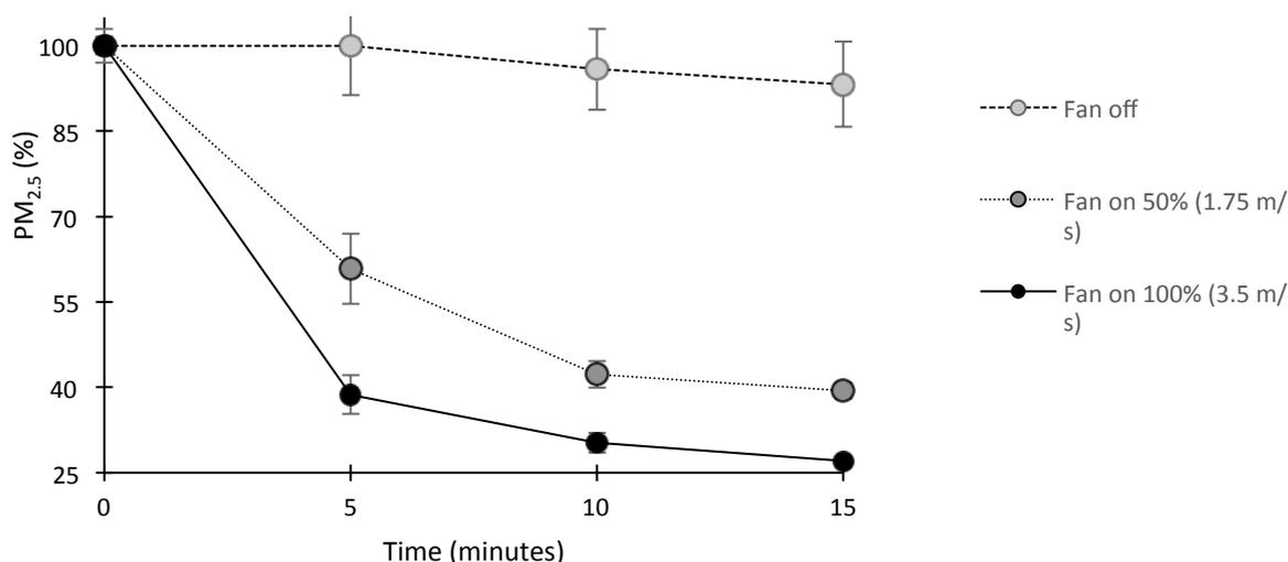
Thus the Breathing Wall modules are extremely efficient at PM removal when the fans are in operation, especially at the higher tested input velocity of  $3.5 \text{ m.s}^{-1}$ .
